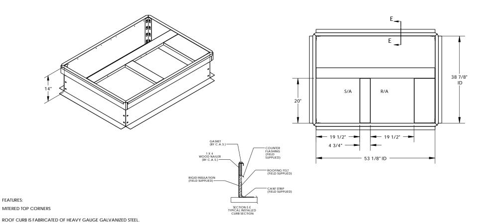
PRE-PUNCHED ASSEMBLY HOLES AND HARDWARE INCLUDED FOR DUCT SUPPORT INSTALLATION,
