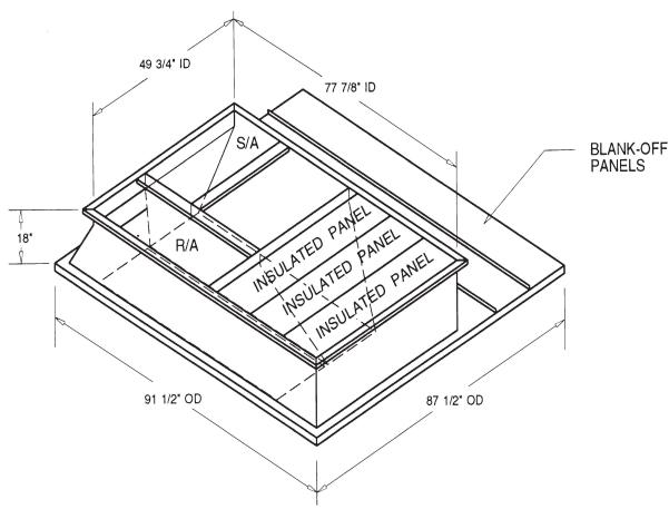
ONE PIECE WELDED CONSTRUCTION
