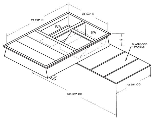
ONE PIECE WELDED CONSTRUCTION
