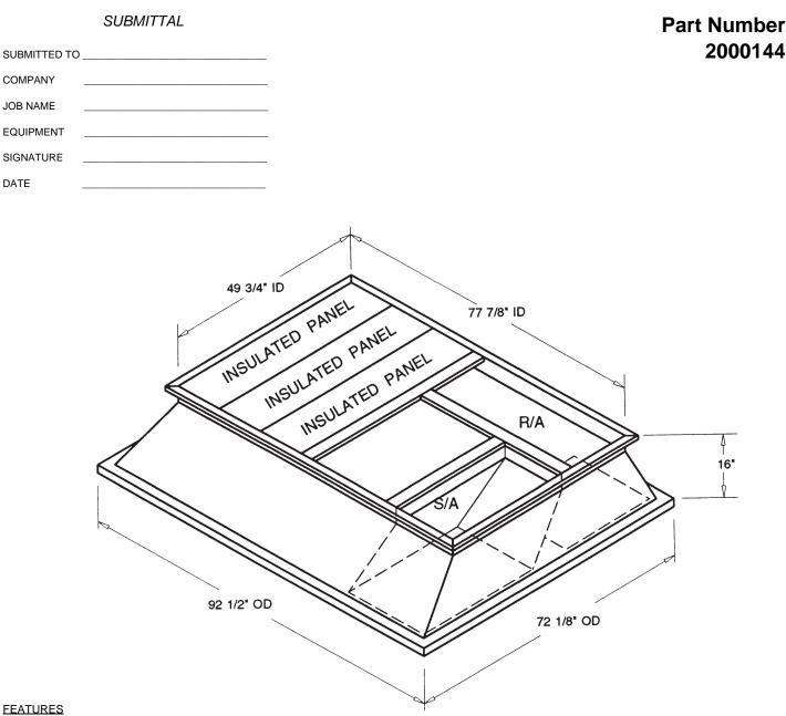
ONE PIECE WELDED CONSTRUCTION
