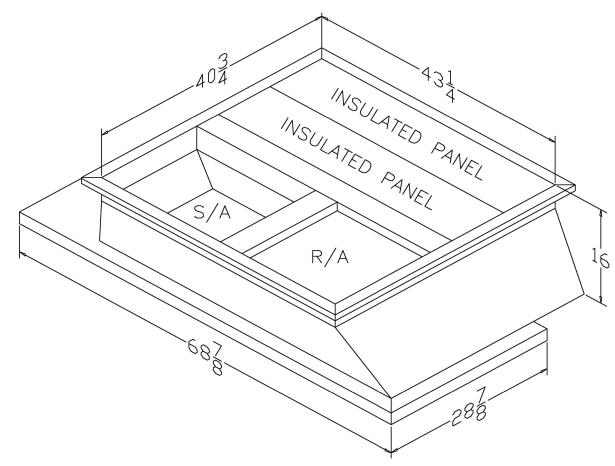
ONE PIECE WELDED CONSTRUCTION
