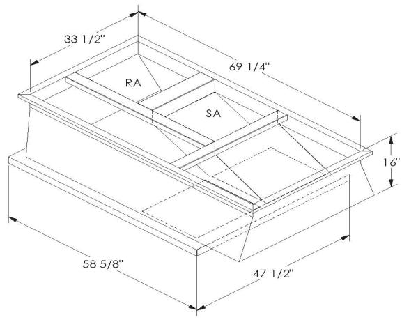
ONE PIECE WELDED CONSTRUCTION
