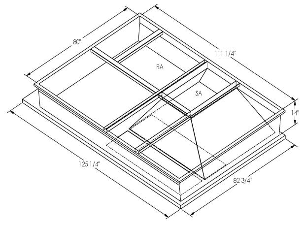
ONE PIECE WELDED CONSTRUCTION
