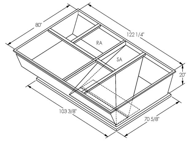
ONE PIECE WELDED CONSTRUCTION
