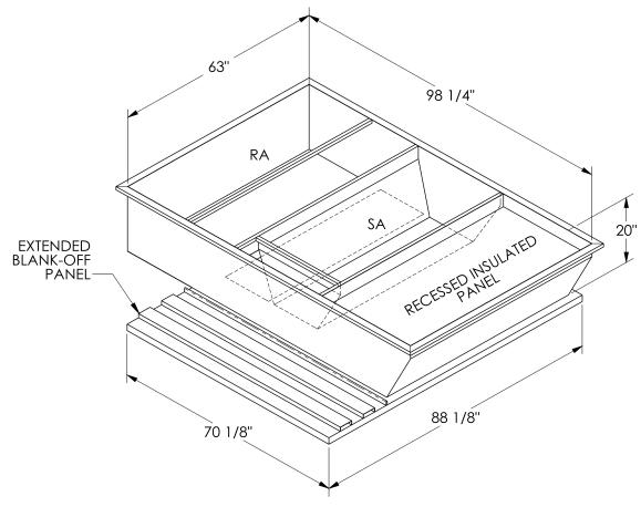
ONE PIECE WELDED CONSTRUCTION
