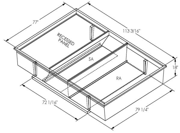
ONE PIECE WELDED CONSTRUCTION
