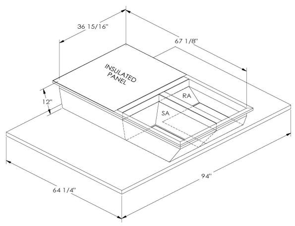
ONE PIECE WELDED CONSTRUCTION
