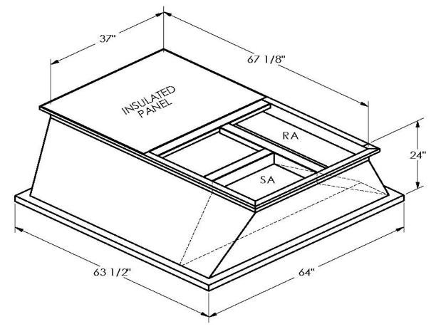
ONE PIECE WELDED CONSTRUCTION
