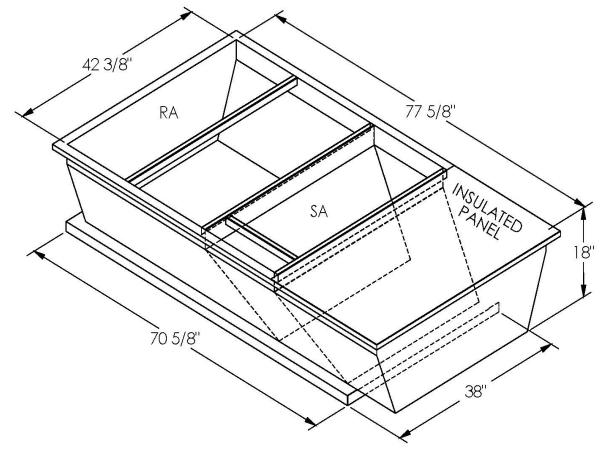
ONE PIECE WELDED CONSTRUCTION
