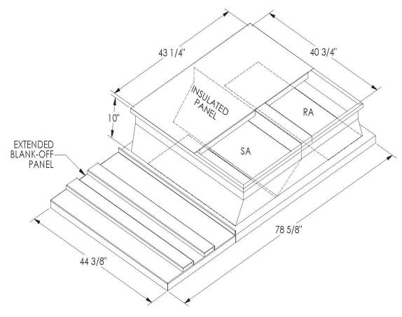
ONE PIECE WELDED CONSTRUCTION
