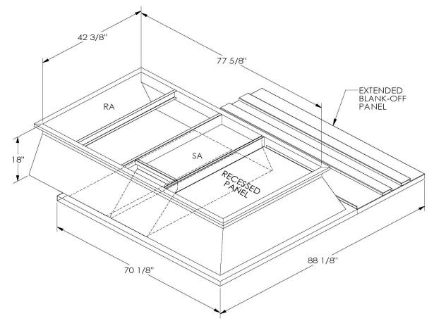
ONE PIECE WELDED CONSTRUCTION
