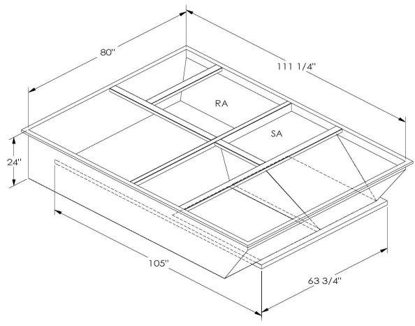
ONE PIECE WELDED CONSTRUCTION
