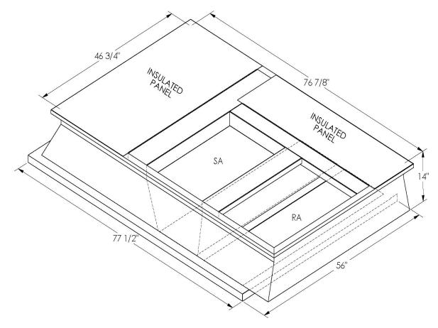
ONE PIECE WELDED CONSTRUCTION
