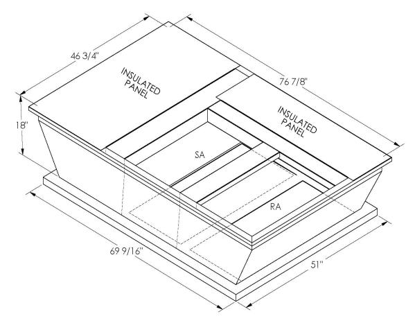
ONE PIECE WELDED CONSTRUCTION
