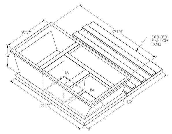
ONE PIECE WELDED CONSTRUCTION
