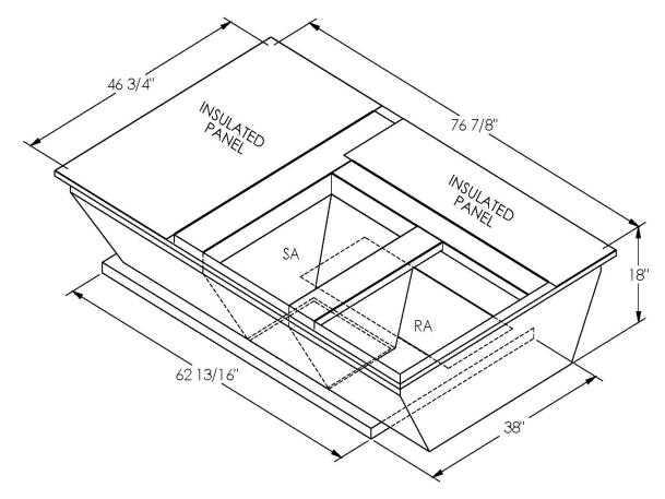
ONE PIECE WELDED CONSTRUCTION
