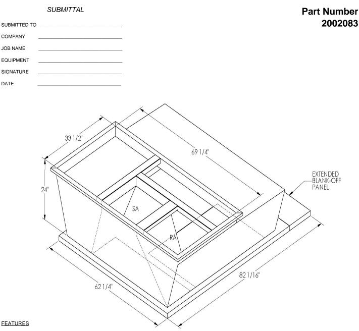
ONE PIECE WELDED CONSTRUCTION
