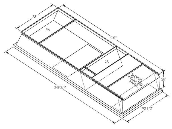
ONE PIECE WELDED CONSTRUCTION
