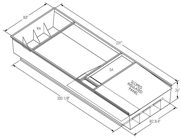
ONE PIECE WELDED CONSTRUCTION
