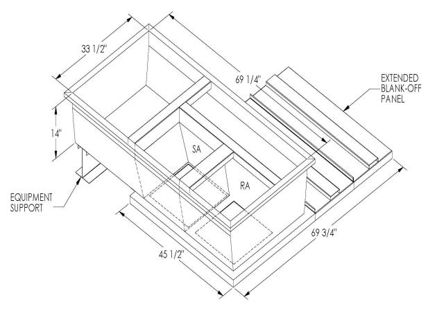
ONE PIECE WELDED CONSTRUCTION
