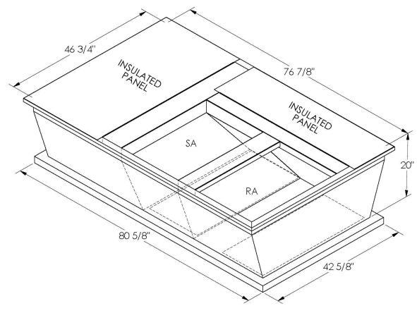
ONE PIECE WELDED CONSTRUCTION
