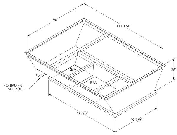
ONE PIECE WELDED CONSTRUCTION
