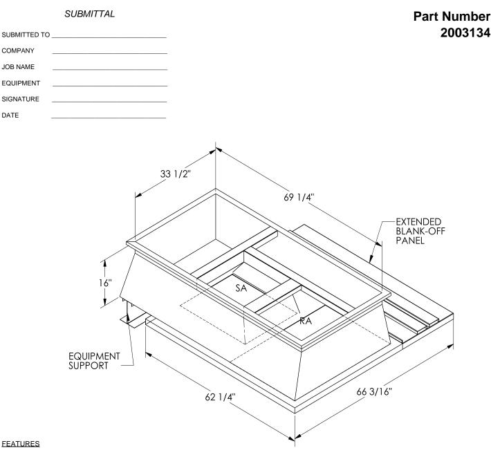
ONE PIECE WELDED CONSTRUCTION
