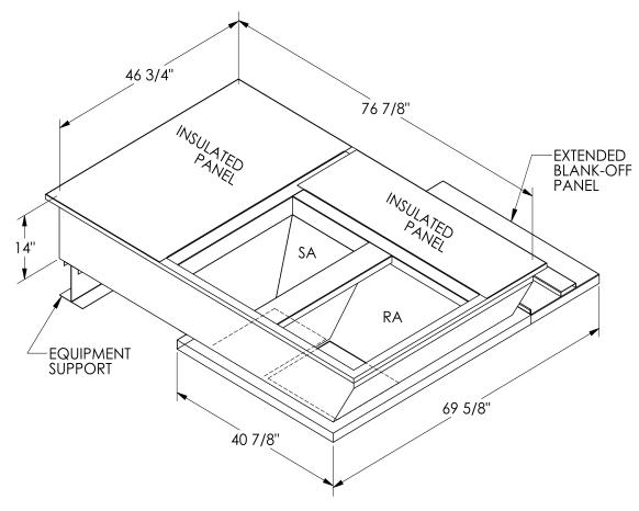
ONE PIECE WELDED CONSTRUCTION
