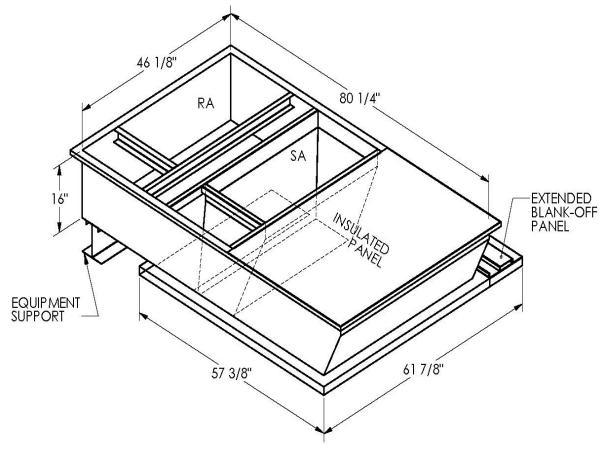
ONE PIECE WELDED CONSTRUCTION
