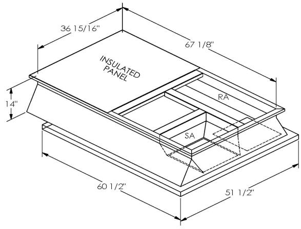
ONE PIECE WELDED CONSTRUCTION
