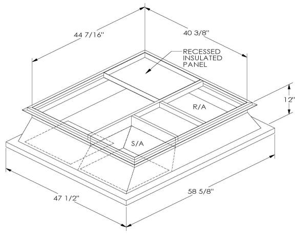
ONE PIECE WELDED CONSTRUCTION
