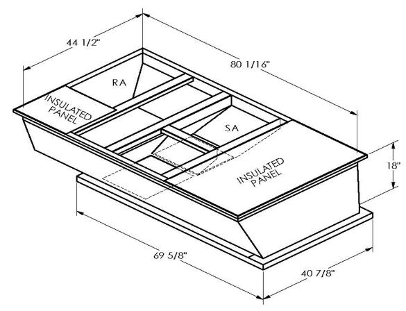
ONE PIECE WELDED CONSTRUCTION
