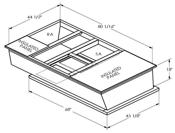
ONE PIECE WELDED CONSTRUCTION
