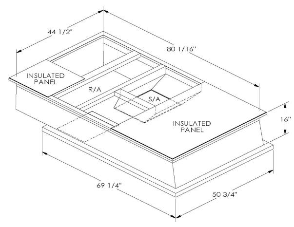
ONE PIECE WELDED CONSTRUCTION
