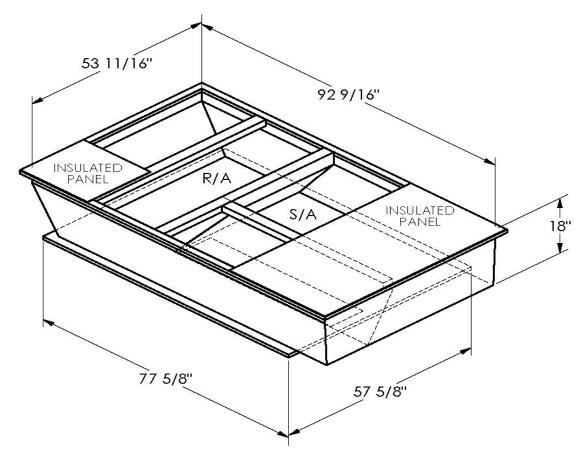
ONE PIECE WELDED CONSTRUCTION
