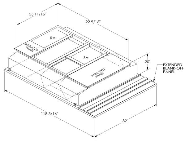
ONE PIECE WELDED CONSTRUCTION
