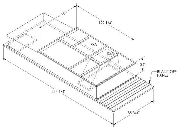
ONE PIECE WELDED CONSTRUCTION
