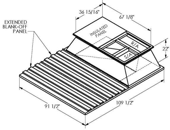
ONE PIECE WELDED CONSTRUCTION
