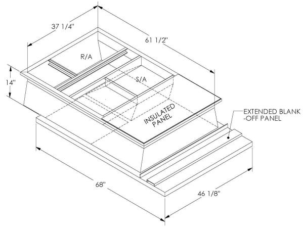
ONE PIECE WELDED CONSTRUCTION
