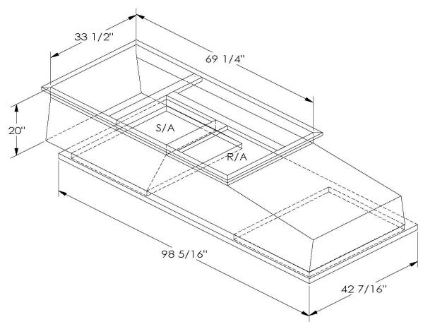
ONE PIECE WELDED CONSTRUCTION
