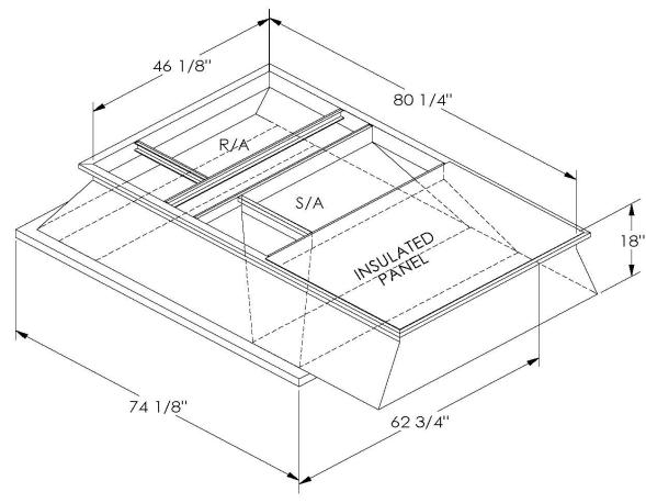
ONE PIECE WELDED CONSTRUCTION
