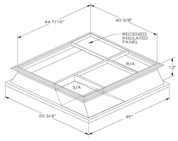
ONE PIECE WELDED CONSTRUCTION
