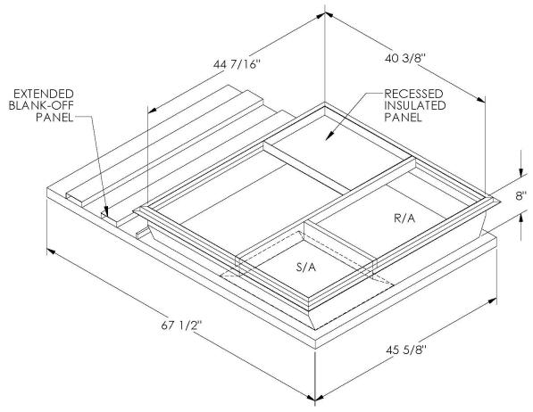
ONE PIECE WELDED CONSTRUCTION
