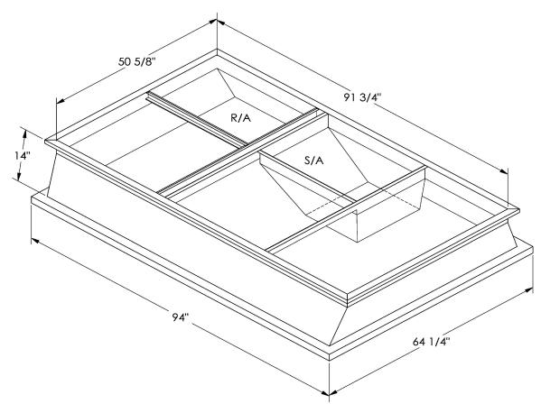
ONE PIECE WELDED CONSTRUCTION
