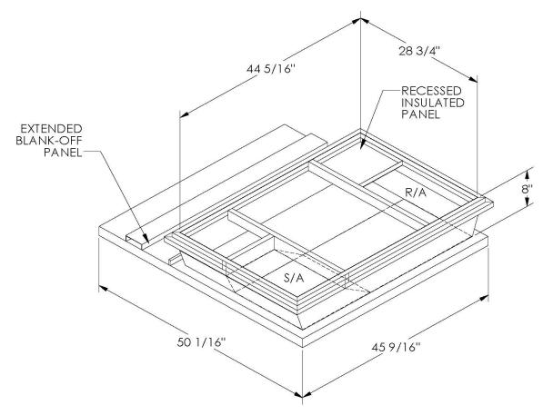
ONE PIECE WELDED CONSTRUCTION
