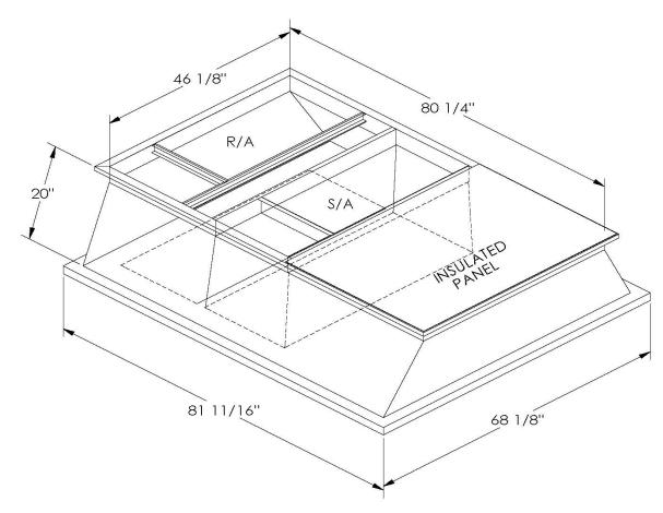
ONE PIECE WELDED CONSTRUCTION
