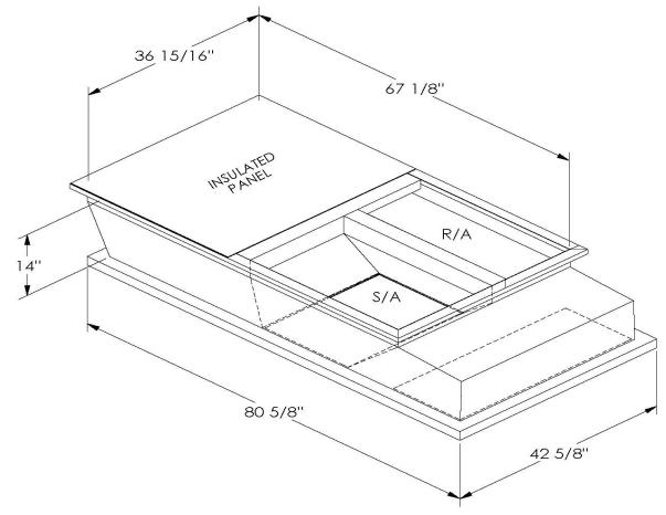
ONE PIECE WELDED CONSTRUCTION
