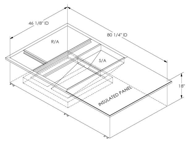
ONE PIECE WELDED CONSTRUCTION
