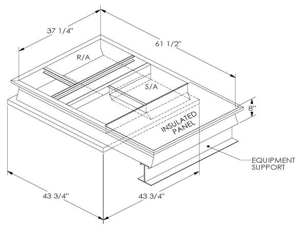
ONE PIECE WELDED CONSTRUCTION
