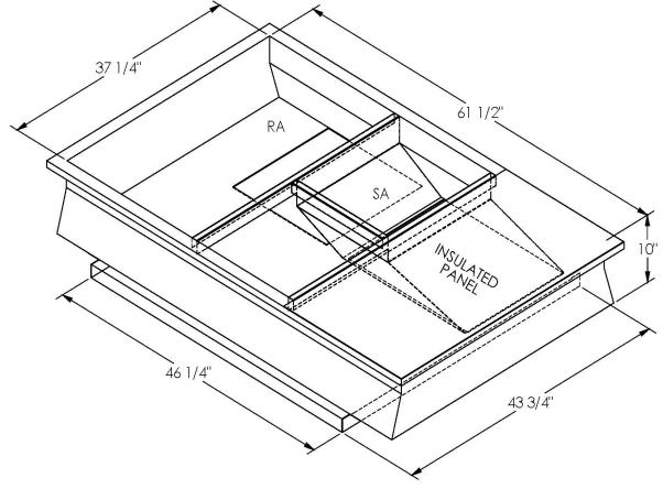
ONE PIECE WELDED CONSTRUCTION
